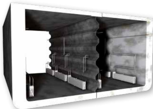
*PLATECOIL®-based cargo heating system in articulated tug barges. The drawing is not to scale; banks and piping are enlarged for clarity.*
