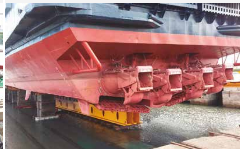
LIFTING PLATFORM OF 175 M LONG AND 30 M WIDE, UP TO 10,000 TONS LIFTING CAPACITY (FOR VESSELS UP TO 36,000 DWT)
